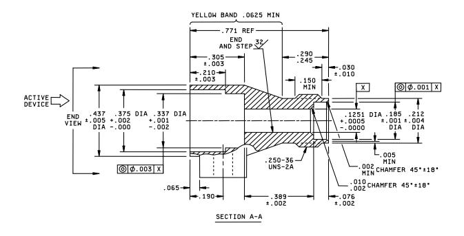
FIGURE 1. <u>Dimensions and configuration</u>.
